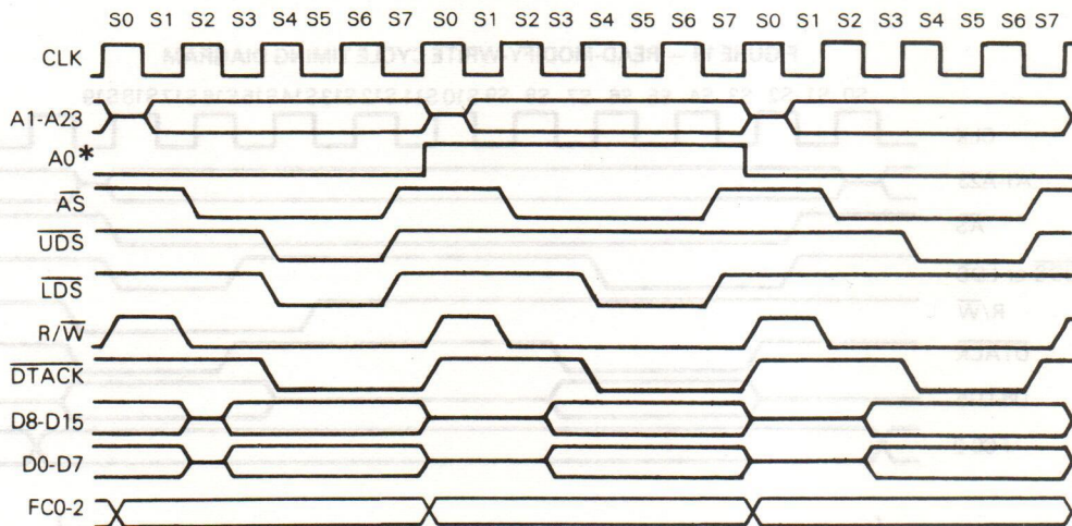
FIGURE 17 — WORD AND BYTE WRITE CYCLE TIMING DIAGRAM
